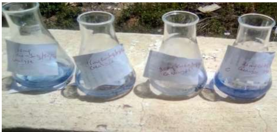
Figure 9.10mg, 15mg, 20mg and 25 mg \text{Cu-SnO}_2/\text{g-C}_3\text{N}_4 nano composite in 30mg MB solution in sun light radiation for 60min
