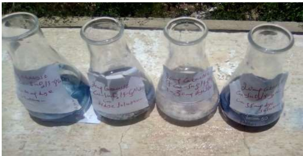
Figure 6.20 mg Cu-SnO 2 /g-C 3 N 4 nano composite in 20 mg, 25 mg, 30 mg and 35 mg MB dye solution in sun light radiation for 60 min
