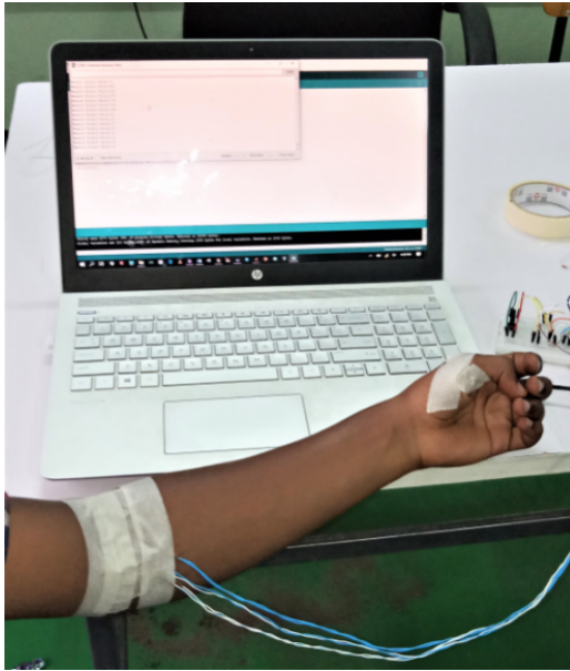
(a) Attaching the strain gauge sensor
