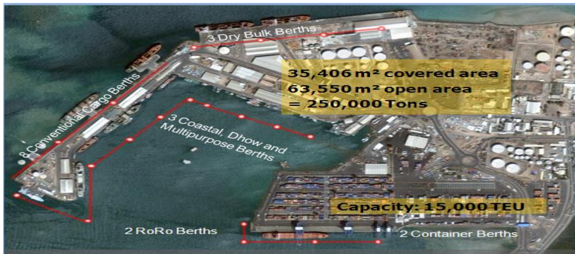
Figure 3.3: Djibouti port structures and layout
