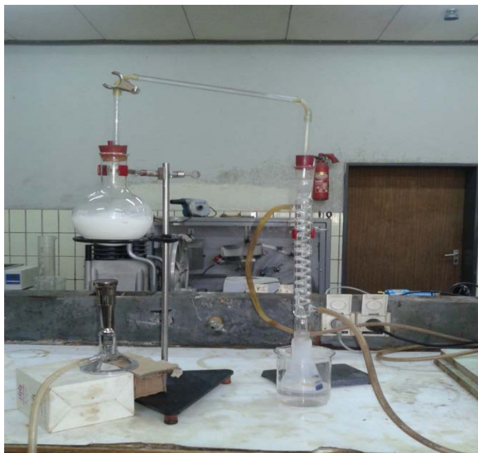
Fig 3.2 Experimental set up for ammonium chloride determination
