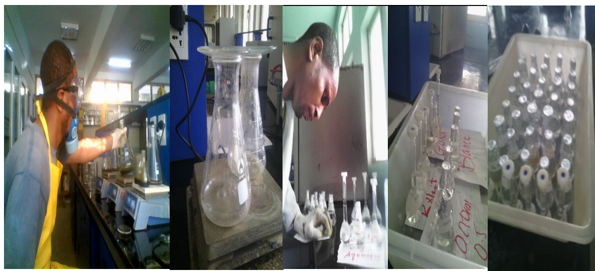
Fig.2. Digestion of soil using hotplate and standard preparation for AAS
