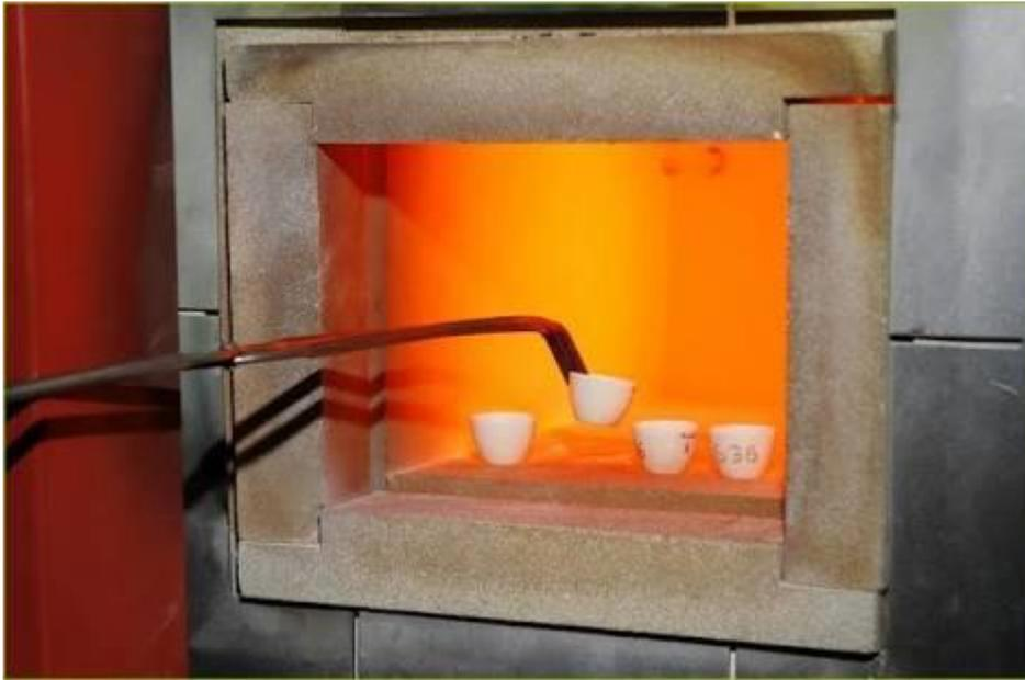
Figure 3 Muffle Furnace or Carbonation to decompose BA sample
