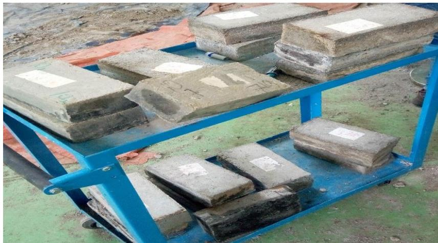
Figure 13 Produced cementitious brick block
