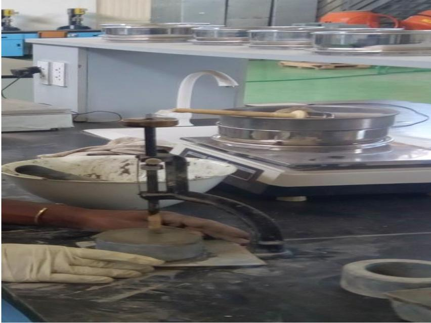
Figure 5 Consistency taste of blended mortar paste AASTU laboratory
