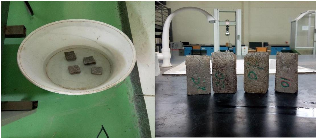
Figure 12 Specimen immersion for water absorption of mortar taste.
