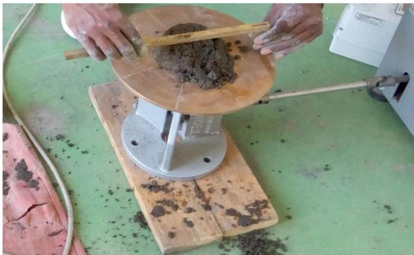
Figure 8 Workability taste for blended mortar paste AASTU construction laboratory
