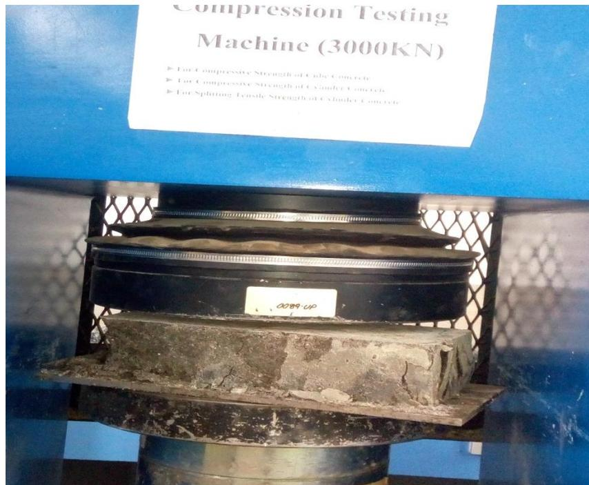
Figure 11 Compressive strength of cementitious brick block tests
