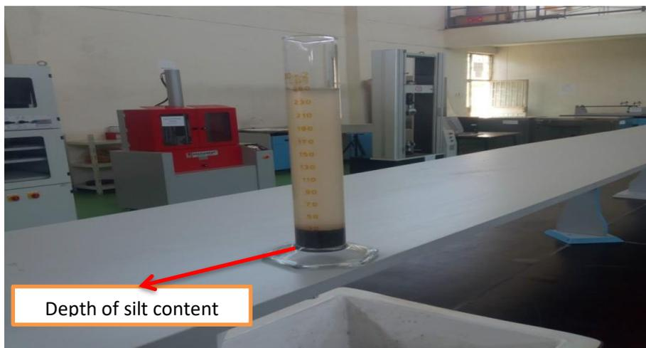
Figure 6 Silt content tastes of fine aggregate taste (sand) AASTU laboratory
