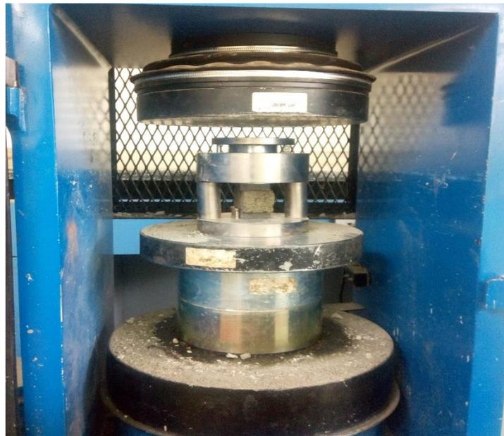
Figure 10 Compressive strength of blended mortar
