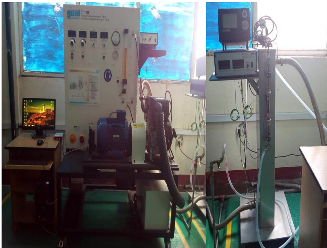
Figure 4-2. Actual setup of the test stand with emission analyzer
