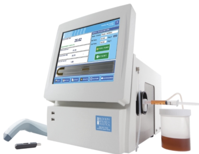
Figure 2-2. DDM 2910 Digital Densitometer, from Rudolf Research
