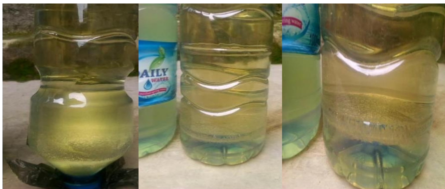
Figure 3-6. Phase separation of the blends prepared before fractional distillation
