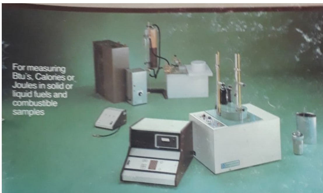
Figure 2-1. Bomb calorimeter setup
