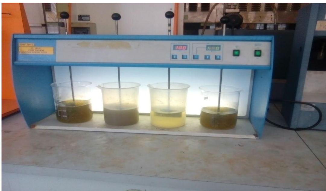
Figure 3. 5: Photographic representation of experimental set up of Jar test apparatus
