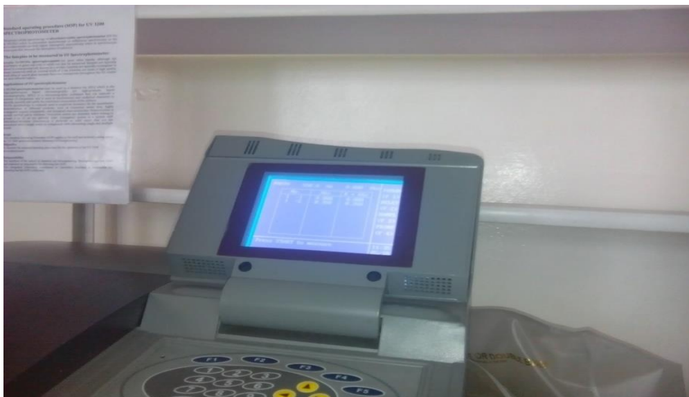
J. Spectro uv-vis Double beam Pc (UVD 3200 model) for color measurement
