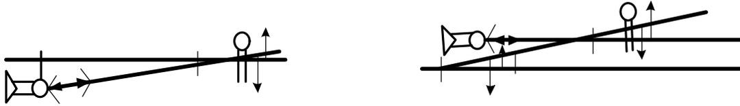
Figure 4.14 One span anchoring
