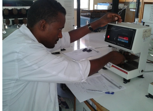
Physical test for dyed crust leathers
