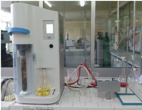
Steam distillation for ammoniac nitrogen estimation
