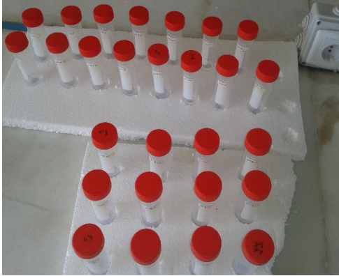
Sample dehydration for microstructure analysis
