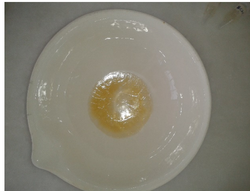
CH drying for solid content estimation
