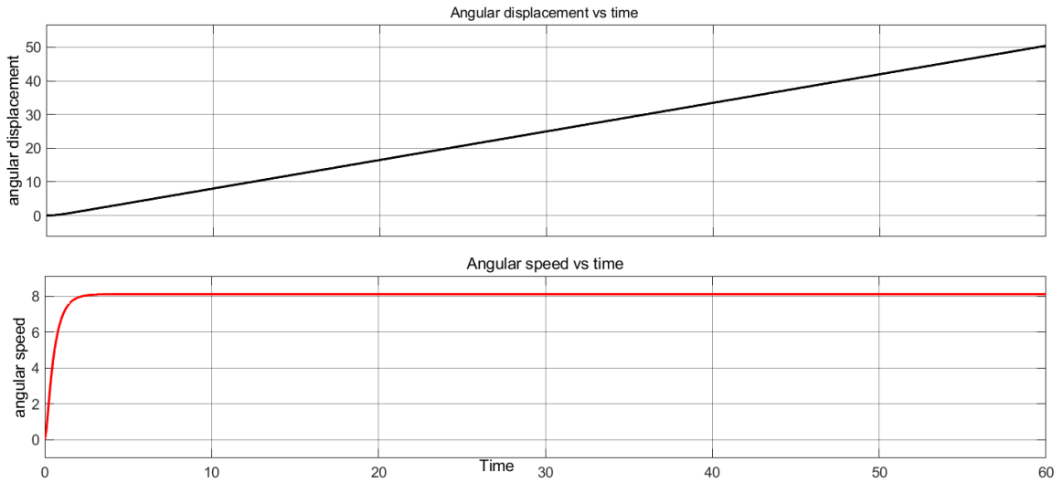
Figure 3.9: Angular displacement and angular speed of the driving motor.
