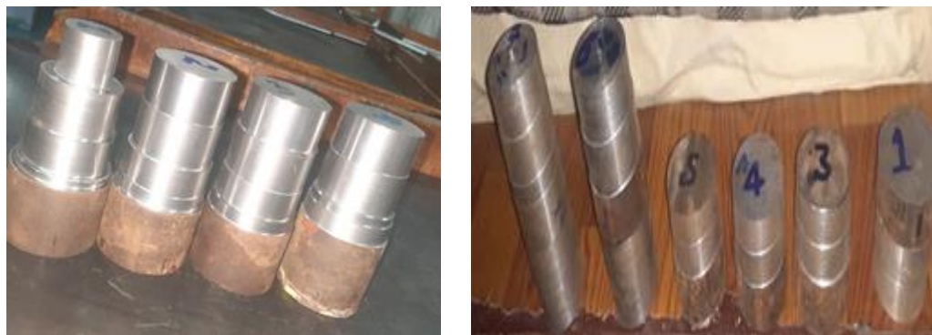
Figure 3. 2: The round AISI 1060 steel sample
