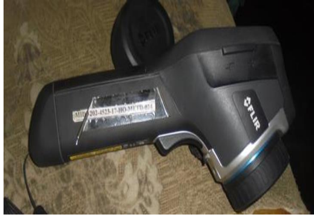
Figure 3. 8: The thermal Camera used for measurement of temperature at cutting zone.
