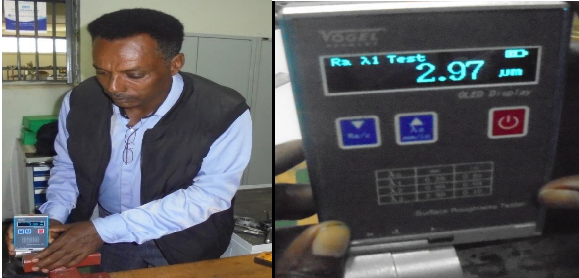
Figure 3. 7: The surface roughness testing procedure
