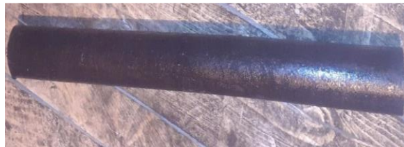
Figure 3. 1: The round AISI 1060 steel bar prepared before cut into specimen for each experimental run.
