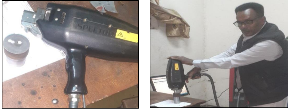
Figure 3. 4: The Spectro test conducted for the Sample
