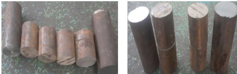
Figure 3. 2: The round AISI 1060 steel sample
