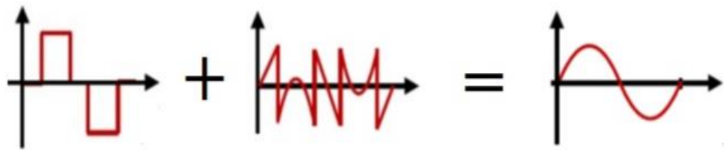
Figure 4.1 : working principle of SAPF
