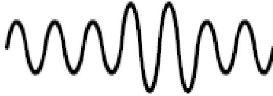
Figure 2.2 : Diagram of voltage swell
