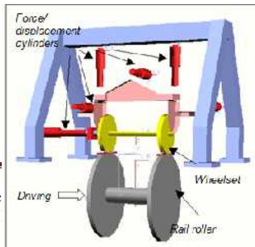
Figure 5: Wheel-rail test rig, schematic [21]
