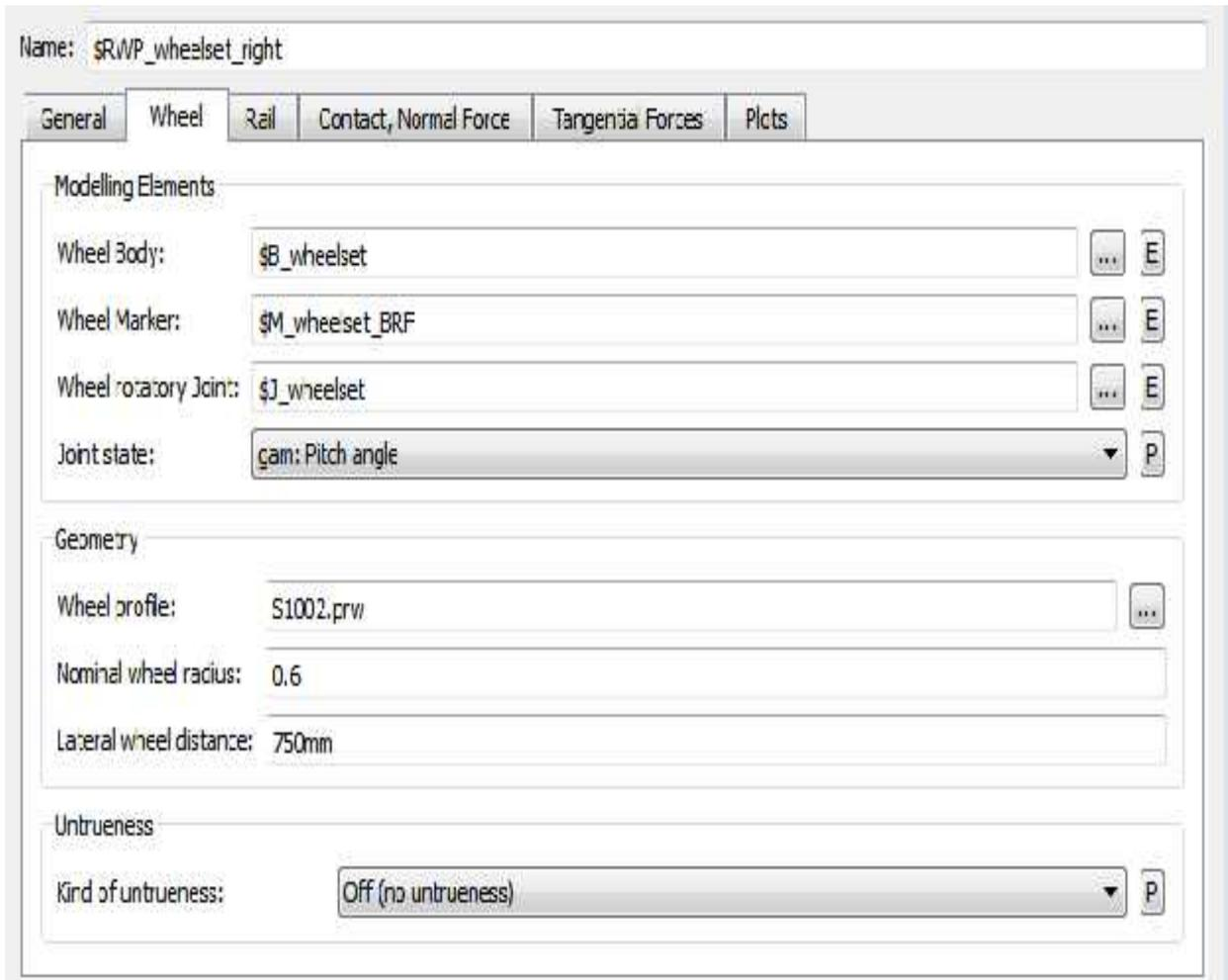
Figure 14: Wheel & Rail properties
