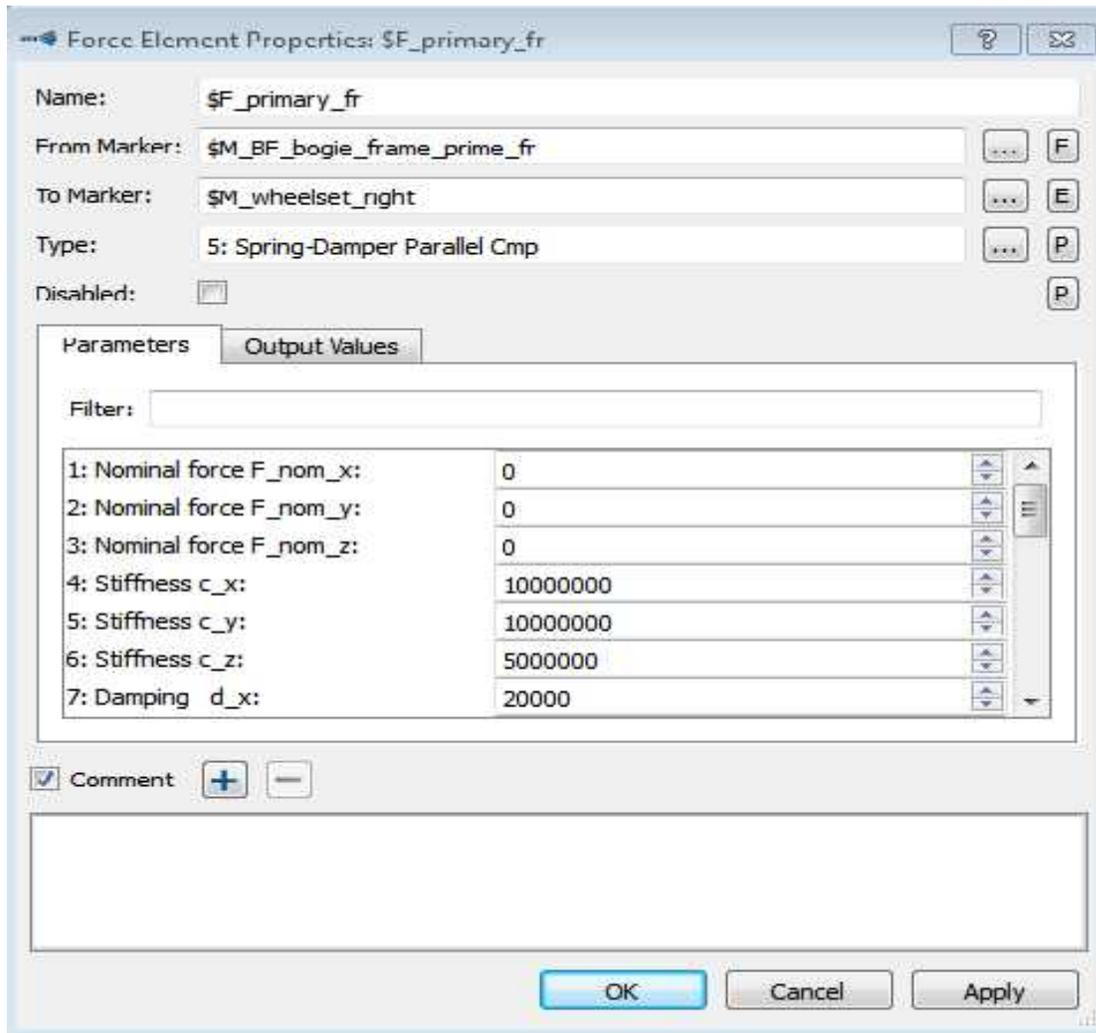
Figure 17: Primary suspension stiffness and damping values
