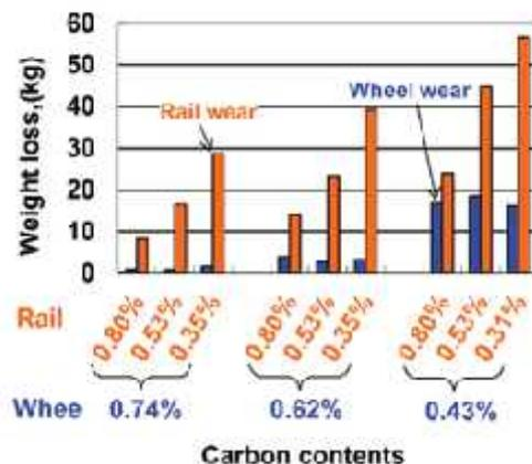
**Figure 4: Carbon content Vs Wear [26]**
