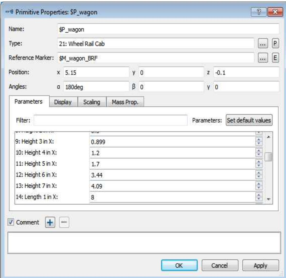
Figure 25: Wagon dimension inputs
