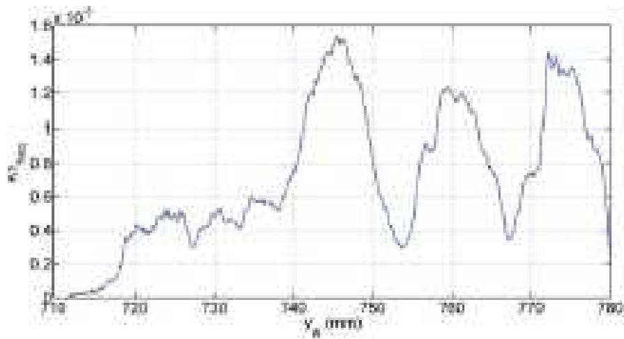
**Figure 10: Typical frequency distribution of the K1 wear regime after taking the average on wheels and simulations [22]**
