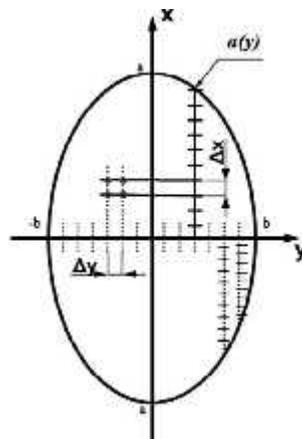
**Figure 8: The contact patch discretization in the FASTSIM algorithm [22]**
