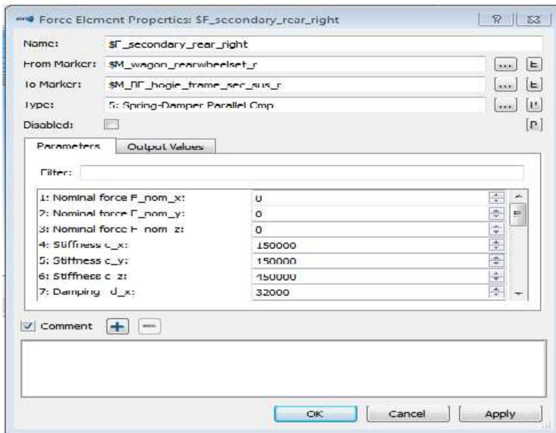
**Figure 18: Secondary suspension**
