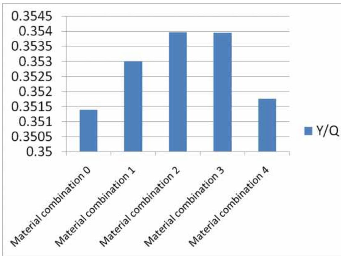
**Figure 32: Maximum derailment coefficient of the five material combinations**
