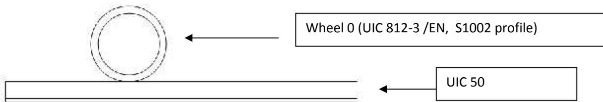
**Figure 26: Explanation of Material combination, example: - Material combination 0**
