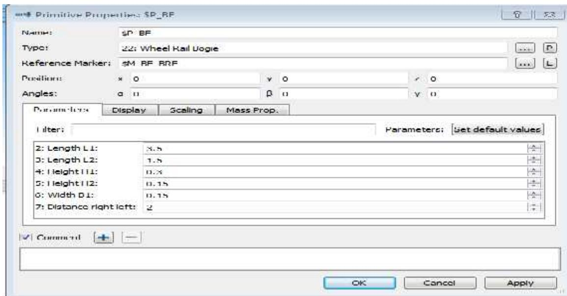
Figure 22: Bogie dimension inputs
