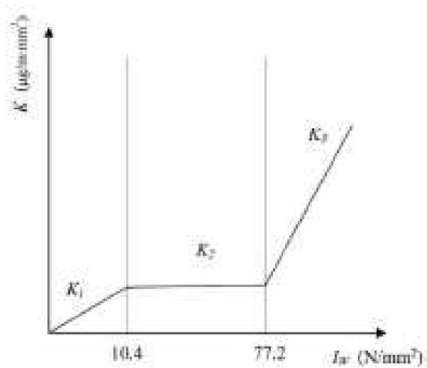
Figure 9: The wear rate as a function of wear index [22]
