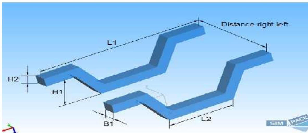
Figure 21: Bogie dimensions
