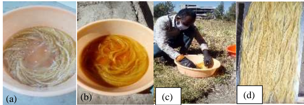
Figure 3- 7. Sisal Fiber Alkali Treatment Process (a) pouring sisal fiber to 5% NaOH solution, (b) sisal fiber treatment for 24 hours, (c) washing the fiber with distilled water, (d) drying the fiber with sun heat
