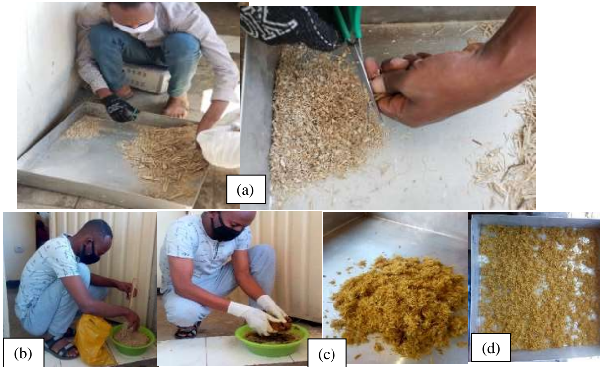
Figure 3- 8. sugar cane bagasse fiber alkali treatment process (a)cutting the SCB fiber into the chopped fiber, (b) pour the chopped SCB fiber into NaOH solution, (c) washing the treated SCB fiber, (e) drying the treated fiber with sun heat.
