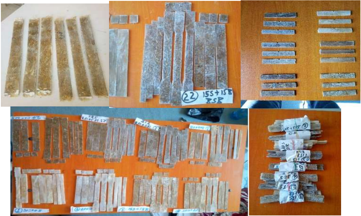
Figure 3- 16. final produced sample specimens which are ready for mechanical test
