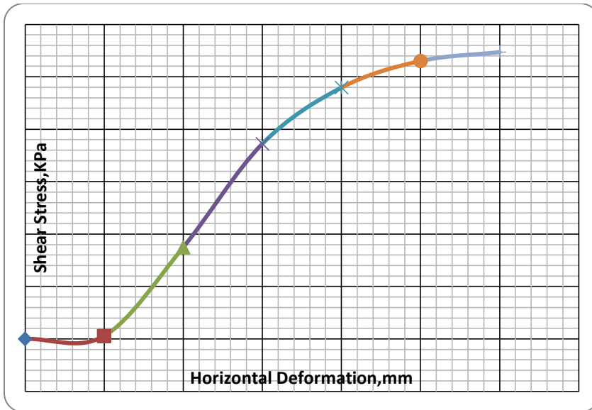
Figure 22 Horizontal deformation Vs Shear stress, Normal stress 81.75 kpa
