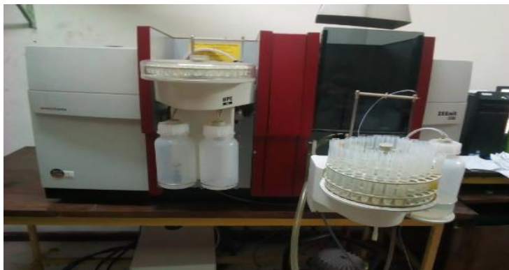
fig 3.8: AAS (Model ZEE Nit 700 P Analytikjena Manufacturing Co. Ltd, Germany)
