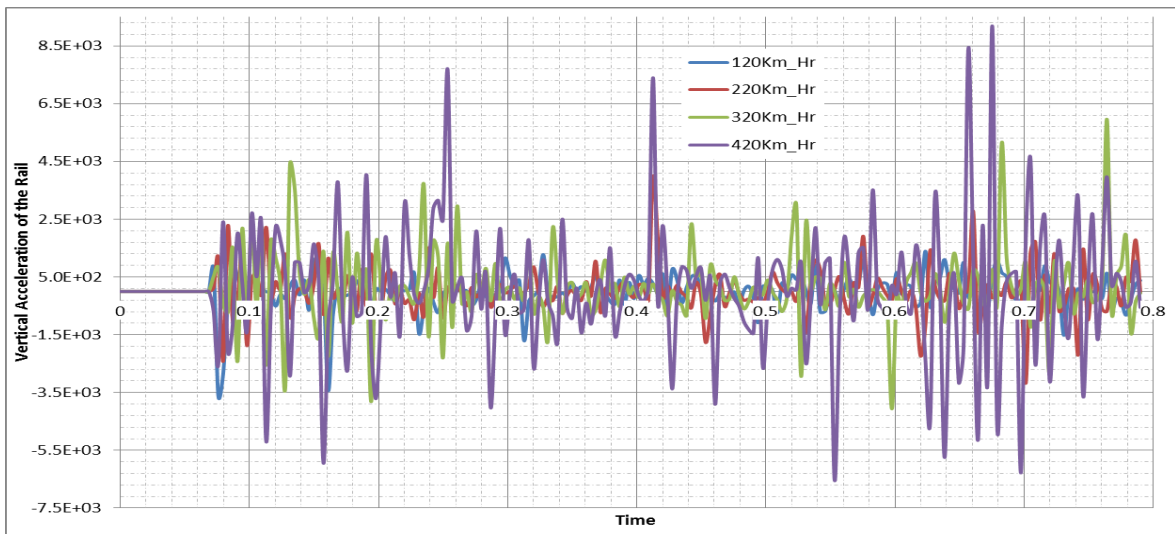
Figure 25: Acceleration of Rail in Rheda2000 Track @ Speed of the wheel at mid of Rail
