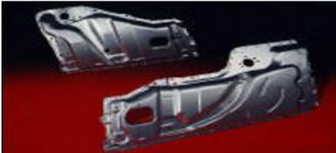
Figure1.9 Automotive structures are formed sheet for parts such as the entire body-in-white.
