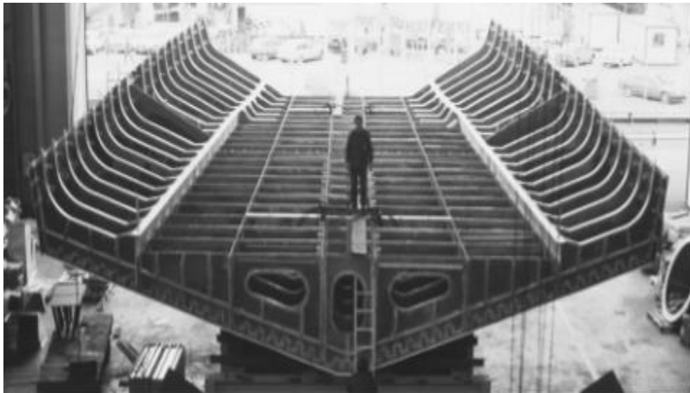
Figure 1.3 The internal hull stiffener structure of the high-speed yacht.
