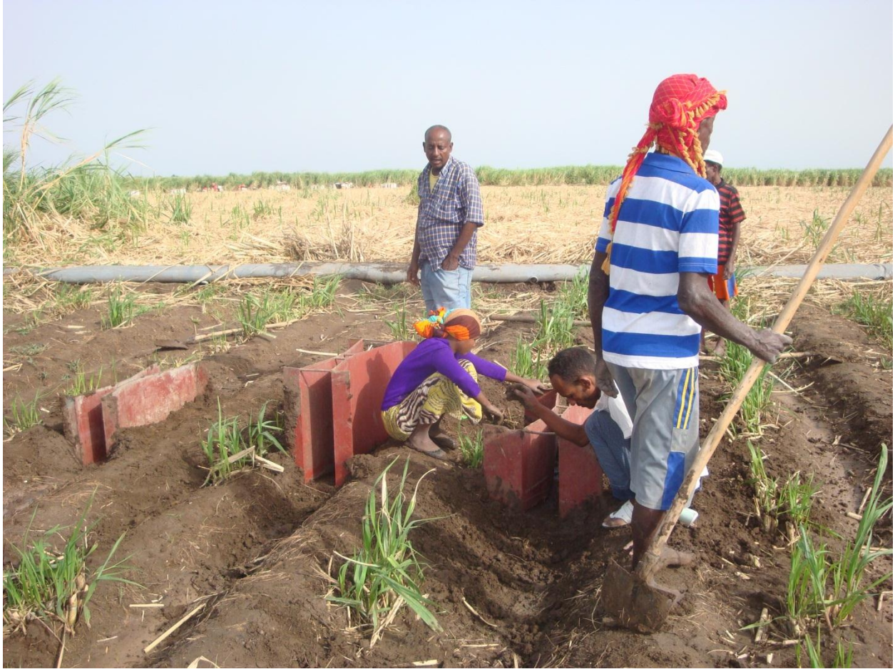
f) Parshall flumes set up to measure furrow inflow rates
