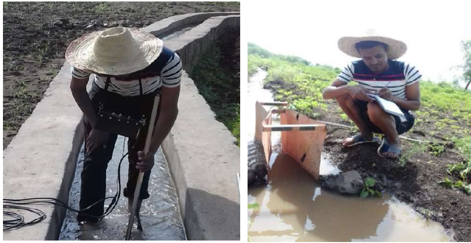
Figure 3.3 Discharge measurement using Current meter and Parshall flume
