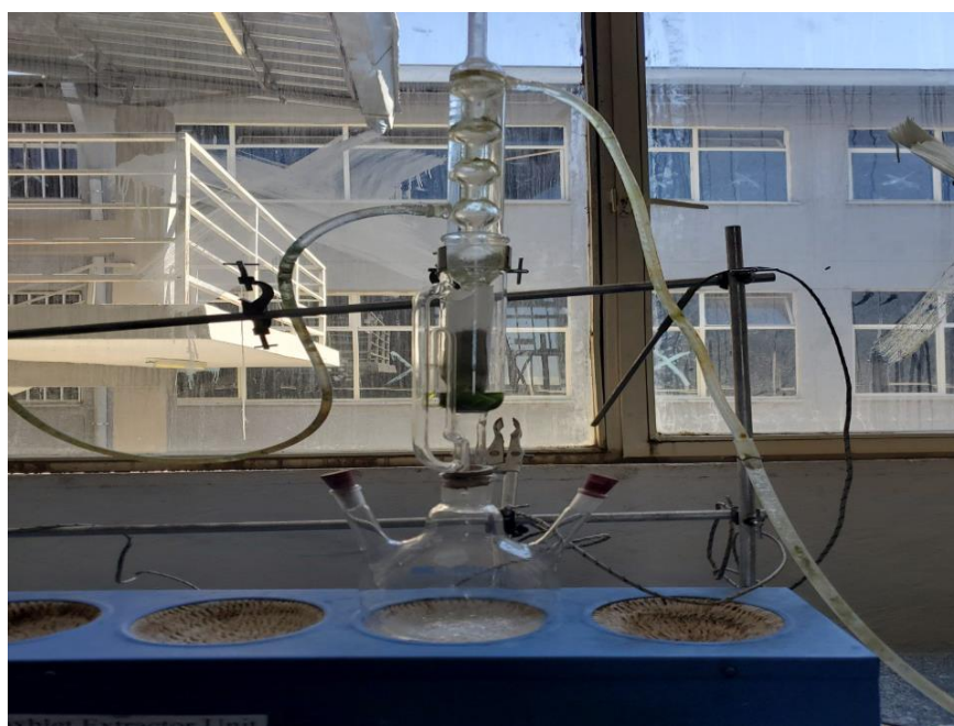
Figure 3. 3. Soxhlet extraction process of extractives
