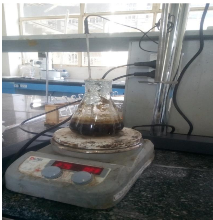
Figure 3. 4. Hemicellulose determination using a hotplate and an Erlenmeyer flask
