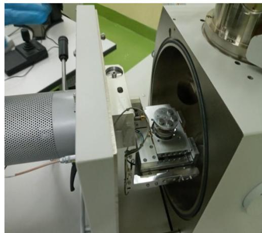
Figure 4. 11 Inserting Powdered Sample to SEM imaging device
