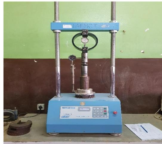
Figure 3. 13 Unconfined compressive test
