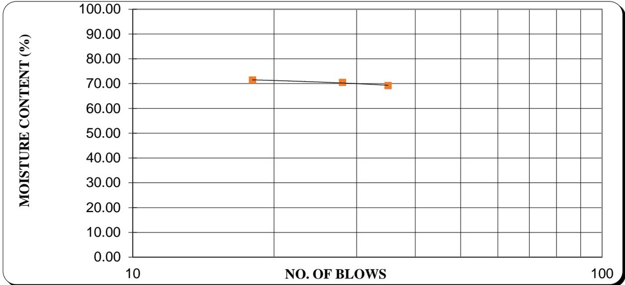
Figure B- 6: Liquid limit chart of 90% BCS with 10% IOT
