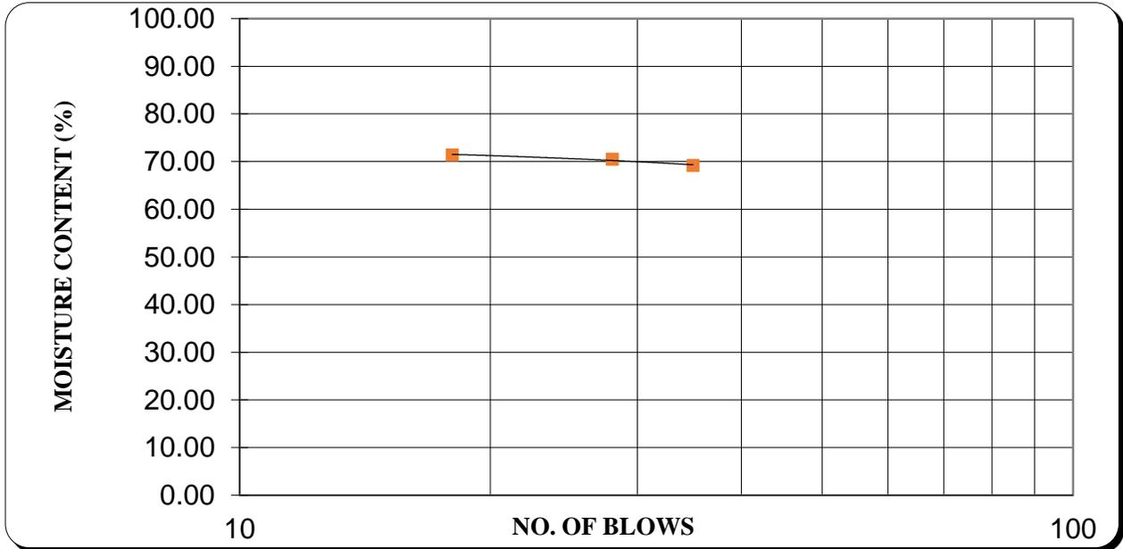
Figure B- 8: Liquid limit chart of 86% BCS with 14% IOT
