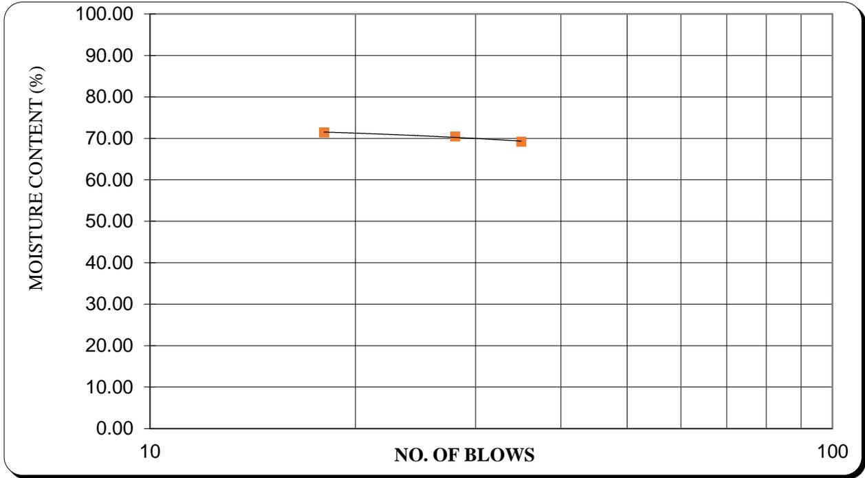
Figure B- 7 Liquid limit chart of 88% BCS with 12% IOT
