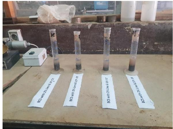
Figure 3. 10 Free swell index test
