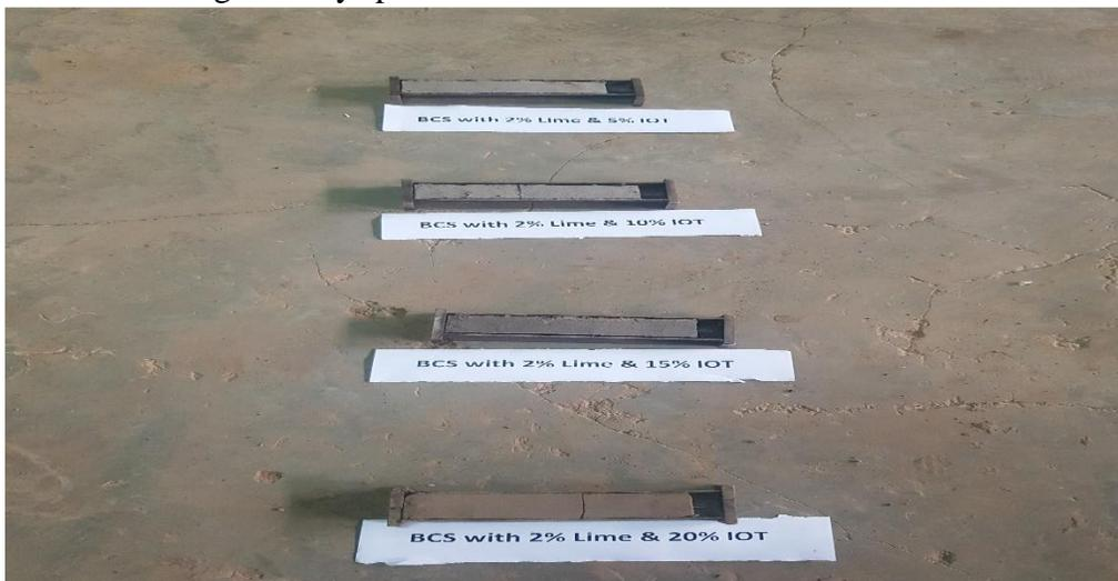
Figure 3. 11 Linear Shrinkage
