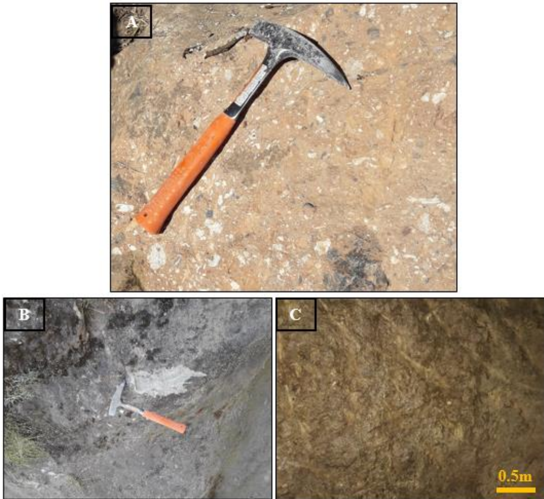
Figure 4. 4: A) highly welded, and unweathered B) unwelded, less weathered, and non-opal bearing and C) unwelded, affected by intense weathering and opal bearing layer of rhyolitic ignimbrite.
